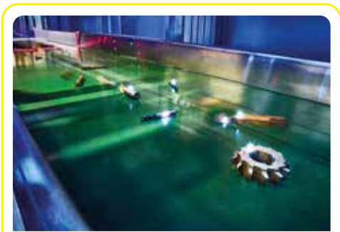
Laser-induced breakdown spectroscopy (LIBS) detects valuable alloys in scrap metal, which recycling robots can then separate by type. This process enables closed-loop material cycles and circumvents downcycling.
