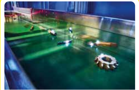
Laser-induced breakdown spectroscopy (LIBS) detects valuable alloys in scrap metal, which recycling robots can then separate by type. This process enables closed-loop material cycles and circumvents downcycling.
